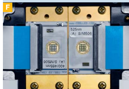
precisExcite: LED array modules
