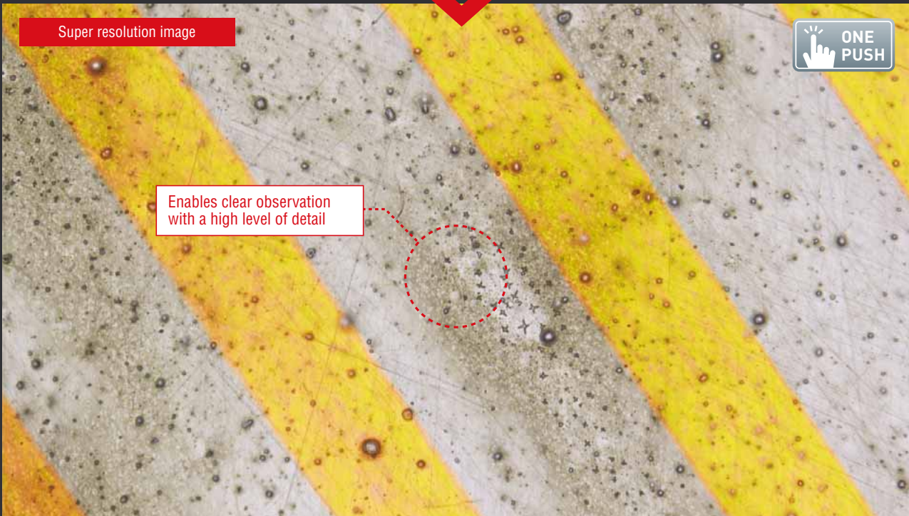
Flexible PC board surface (400x)
