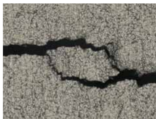
Cracks in stainless steel (300x)
